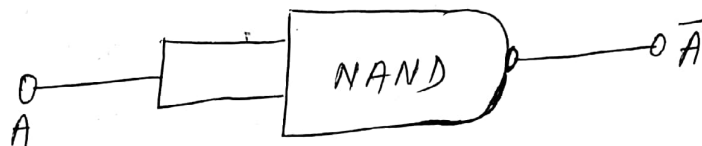
Fig. 6(a) NOT-gate from NAND gate.
